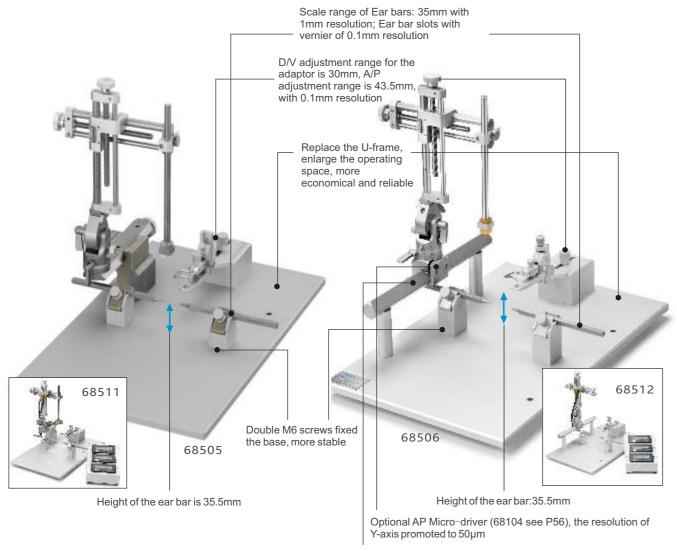
Y-axis slide design, longer moving range:  $\pm$  100mm, 1mm resolution
