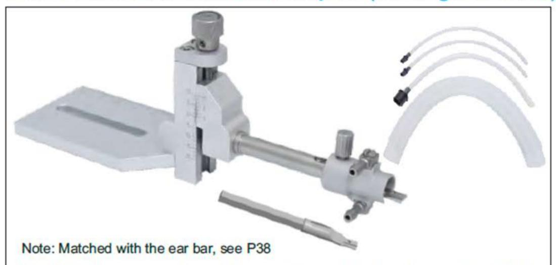
It holds the mouse head by mask and incisor bar, with stable and good effect, and the mask outlet can be connected with the gas evacuation apparatus to evacuate the waste gas and ensure the safety and cleanliness of the operators and the environment.
