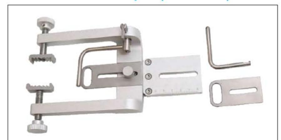
It holds the rabbit head by special malar clamp, adjustable incisor buckle and nose bar. The distance between the two zygomatic clamps can be precisely adjusted by the screw knob.
