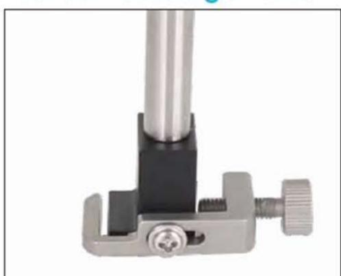
Holder is designed for holding micro amplifier or headstage (Such as TBSI headstage and Plexon microelectrode amplifier). C-shaped head and suitable for diameter from 0.1-7.0mm.
