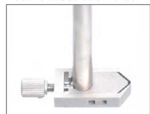
Holder is specifically designed for electrophysiological experiments. Two electrodes, controlled individually, can be located very close to each other. Holds thin electrodes with diameter from 0.7mm to 2.5mm.
