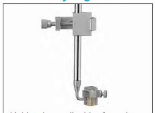
Holder is applicable for microinjection, which holds syringe and needle simultaneously, and the clamping of the syringe is more stable, the syringe holding range is 3mm to 12mm and needle's is 0.3mm to 1.5mm.
