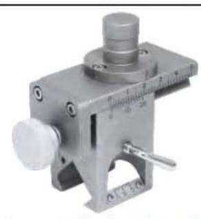
This microdriver can be fine-tuned in the range of 25mm with 50µm step.
