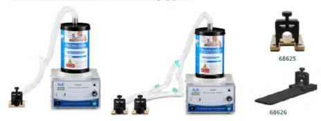
O Simultaneous experiments can be performed on 2–5 rats or mice with five channels of anesthesia mask
