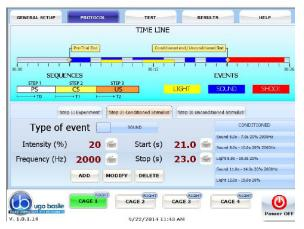
The Unit, incorporating a 12" touch-screen, manages the Passive Avoidance Test via the **40530-010** Software. Up to 4 cages can be connected to the same Controller.
