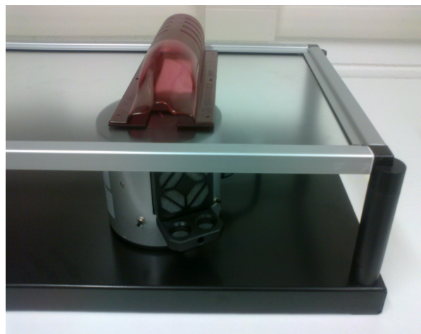
The picture above shows a Durham Holder positioned on a classic Ugo Basile Plantar Test (Hargreaves) device.
