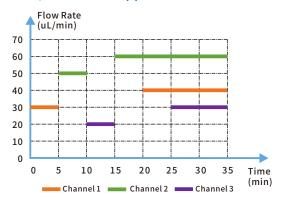
Parameters programming through dedicated PC software can achieve complex flow profiles for four drive units
