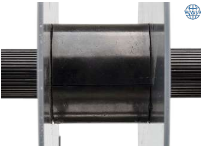
Mouse RotaRod enlarger with rubber (smooth); available also for Rat RotaRod
