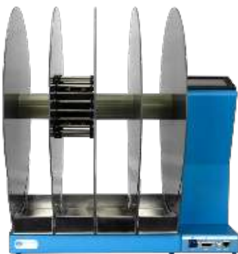
Rat RotaRod with Complex Wheel
