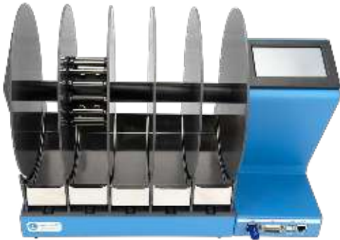
Mouse RotaRod with Complex Wheel
